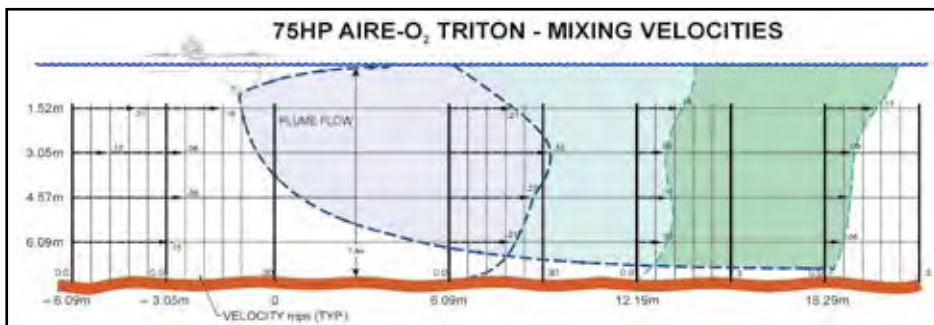
Independent mixing tests on a 75Hp Triton aerator showed velocities out to 60 feet and down to the lagoon's 24 foot depth.
