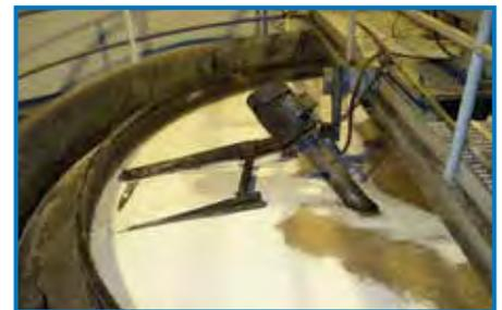
A stream from the pressure vessel is discharged into a separating vessel where the air comes out of solution and is released as a fine bubble spray. These bubbles greatly reduce the pollutants by floating them to the surface where they are removed by equipment designed to remove the floating layer.
